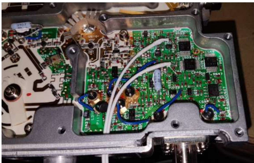
Figure 5: Measurement of phase detector input using thin coax (40Mhz top, 20MHz reference bottom)
