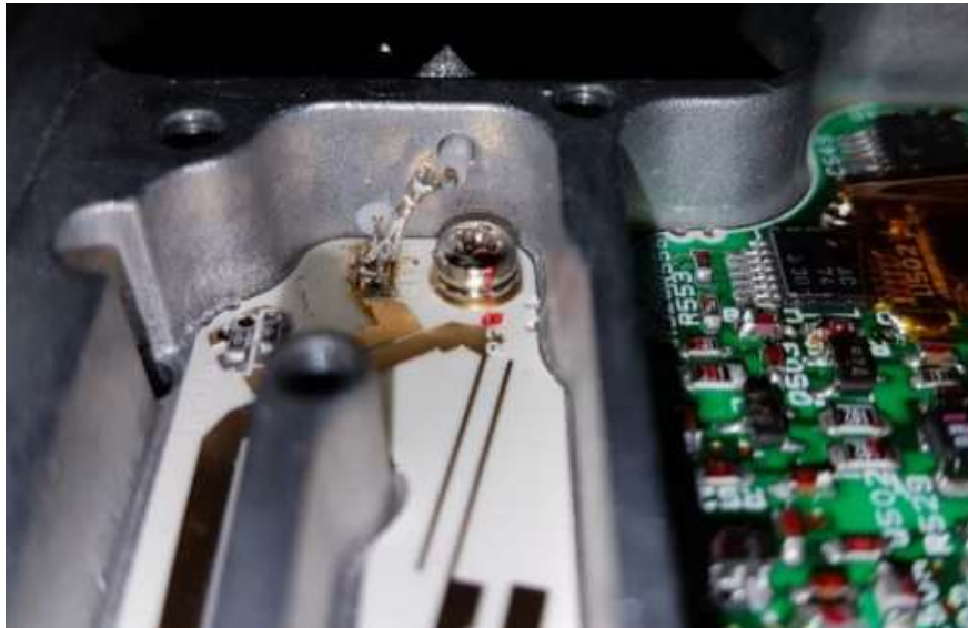
Figure 8: Coax soldered to the stripline
