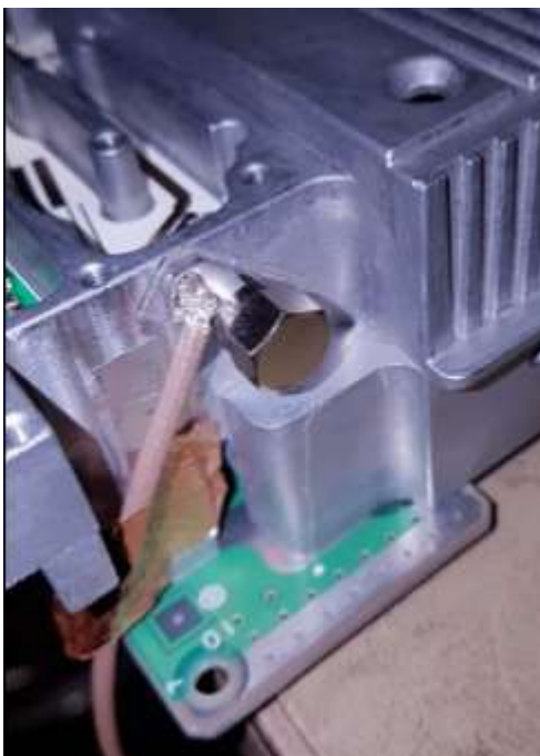
Figure 7: Coax entering the unit
